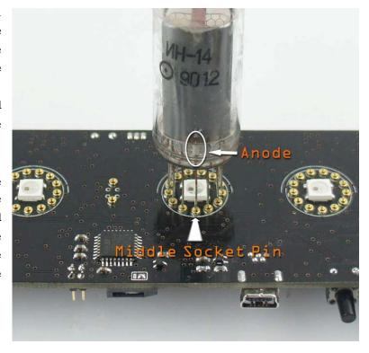
**Note:** In order to protect the socket pins, if not necessary, do not plug /unplug the tube frequently.
