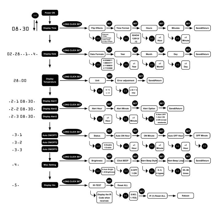
The State Machine of 2-tube NIXIE Clock Vl.O
